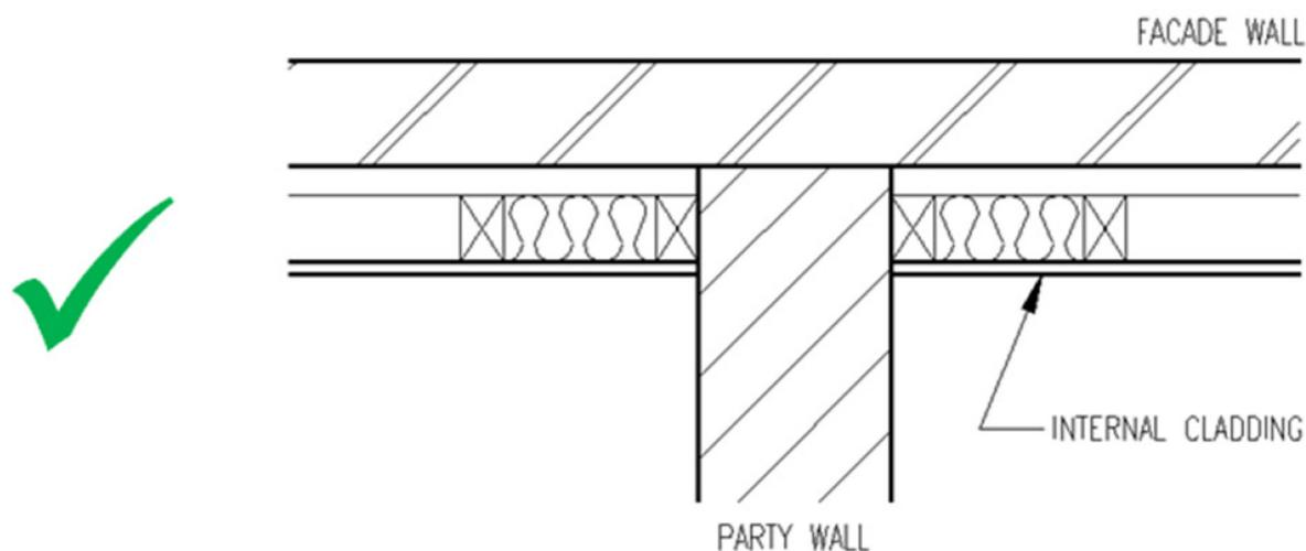
Figure 12 External wall flanking control – Bad design practice
