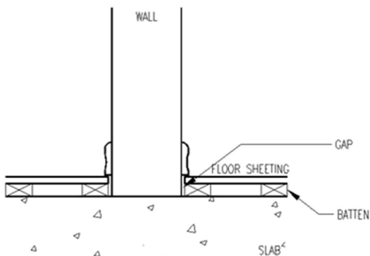
Figure 9 Floor lateral vibration isolation - Bad design practice
