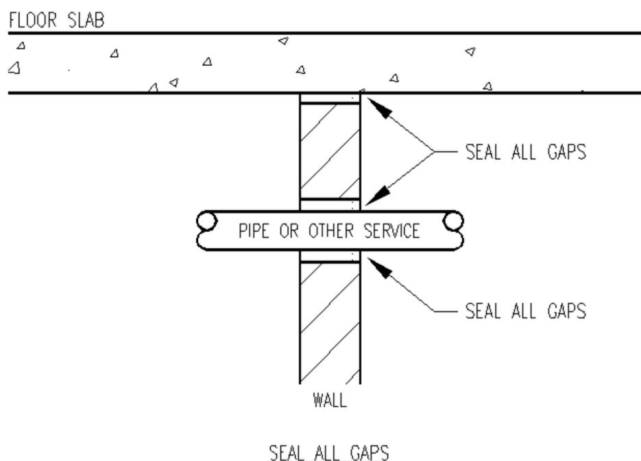
The method of sealing should reflect the environment where the penetration occurs. The seal normally has to remain effective over the life of the building. Sealing is best
