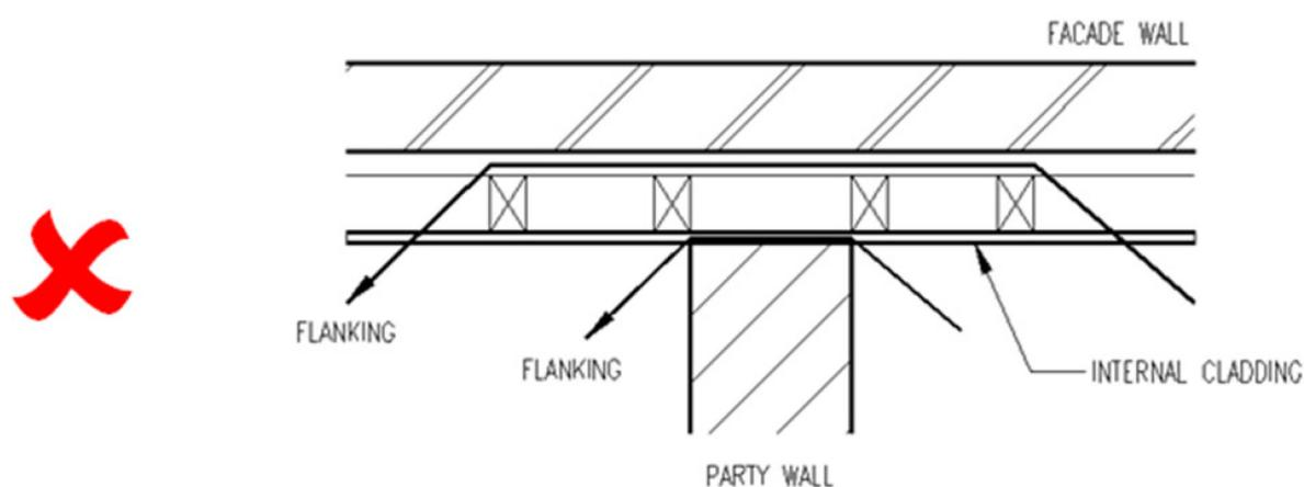
The design measures may need to be applied to the entire façade wall at the time of construction so as to allow suitable flexibility for the location of common walls. For instance, common walls should align at structural columns in the façade where possible and should not be bridged by common air supply grilles or by windows in the façade.
